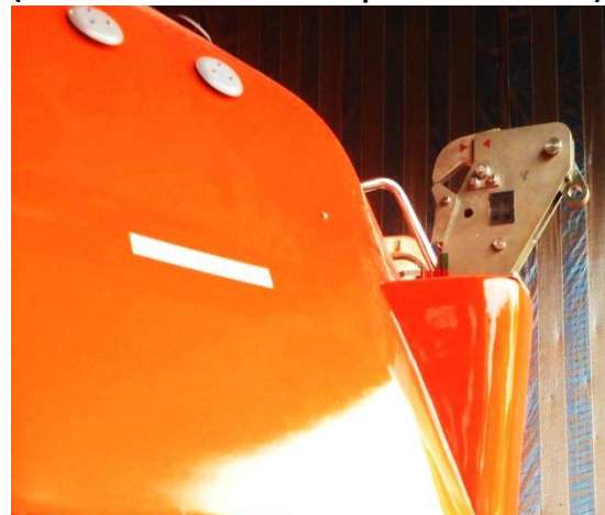
AFTER (retrofitted with IMO compliant Csafe hook)
